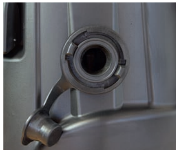
C-pipe connection for wastewater
