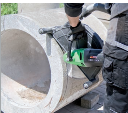
precise cutting depth adjustment (accessory)
