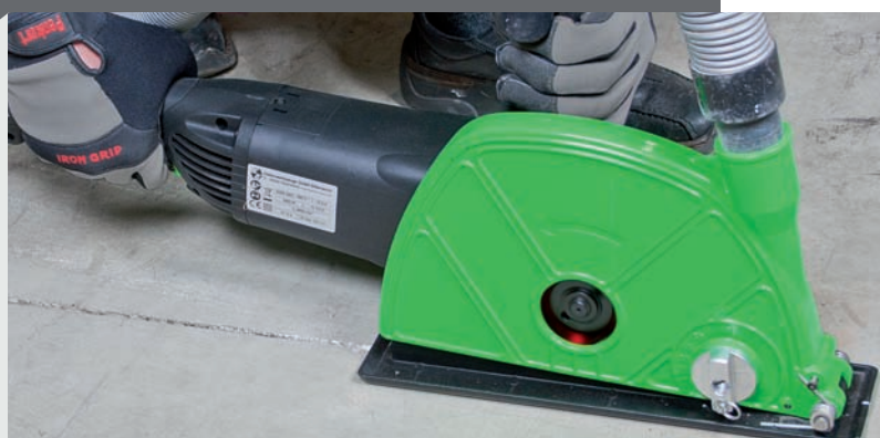
cutting depth adjustment
