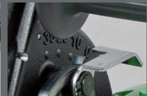
milling depth adjustment
